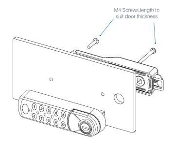
HOLES A & B DIAMETER 4.5 / 5.0mm HOLE D DIAMETER 16.5 / 17mm ALWAYS USE FIXING HOLE A AND HOLE B Recommended screw fixing torque 0.8Nm
