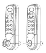
Turn key back 90° to original position and remove from lock
