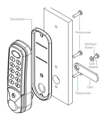
Holes **A**, **B** & **C** diameter 4.5 / 5.0mm Hole **D** diameter 16.0 / 16.5mm Always use fixing hole **A** and either fixing hole **B** or **C** (or both) Recommended screw fixing torque 0.8NM
