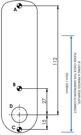
Holes A. B & C diameter 4.5 / 5.0mm Hole D diameter 16.0 / 16.5mm Always use fixing hole **A** and either fixing hole **B** or **C** (or both)
