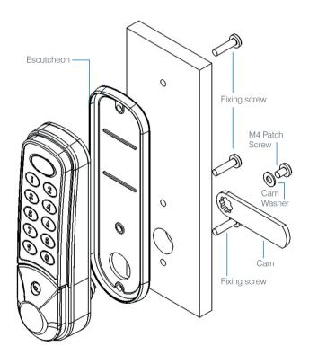
Holes **A**, **B** & **C** diameter 4.5 / 5.0mm Hole **D** diameter 16.0 / 16.5mm Always use fixing hole **A** and either fixing
